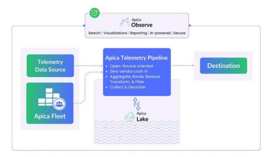
FLOW acts as a central hub, routing data to various destinations like Observability and SIEM tools. It cleans and adjusts data in transit, saving on storage and processing costs.
